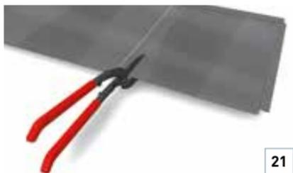
Once the panel has been cut to the required size, turn it over and cut an incision on the back along the fold (see illustration).
