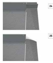
Notch the fold and form an upstand of 20 mm (see Fig. 26 and 27).
