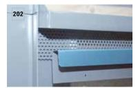
Then, rivet a self-canted channel profile onto the perforated plate (Fig. 201, 202 and 203).
