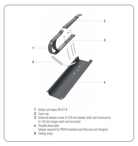
Figure 101 - Safety roof hooks - required material
