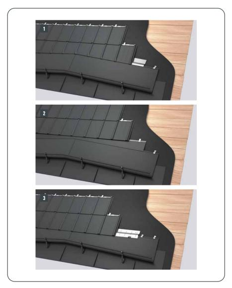
Figure 76 • Joint to an on-roof gutter
